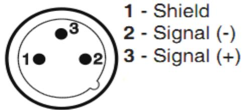
If you are using the standard DMX controllers, you can connect the DMX output of the controller directly with the DMX input of the first fixture in the DMX chain. If you wish want to connect DMX controllers with other XLR outputs, you need to use a dapter-cables.
